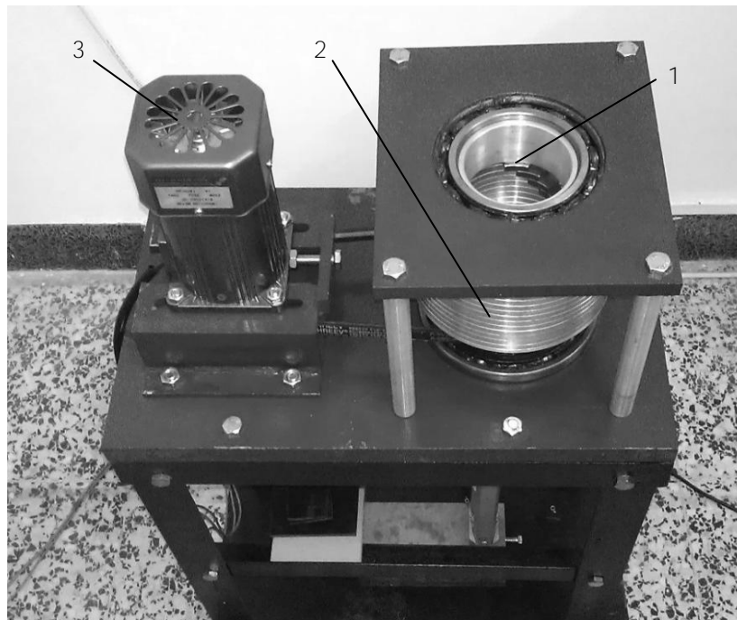
Figure 2. Experimental setup of magnetic stirrer.
