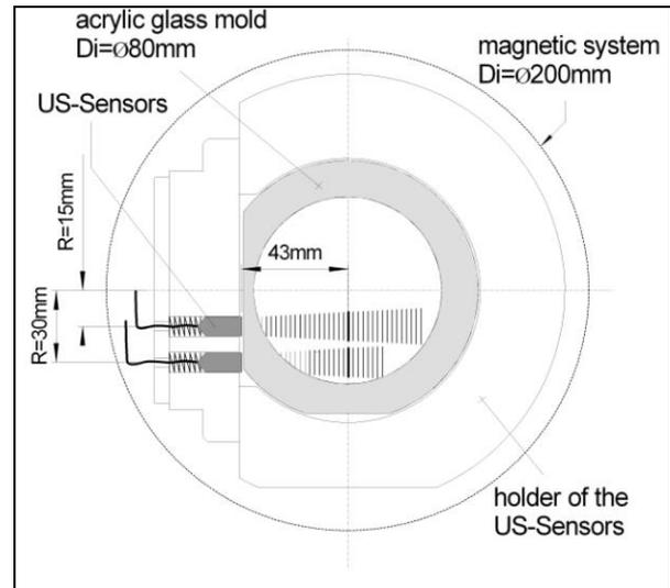
Fig. 2: Horizontal cross section of the mold showing the radial measuring positions 15 mm 30 mm
