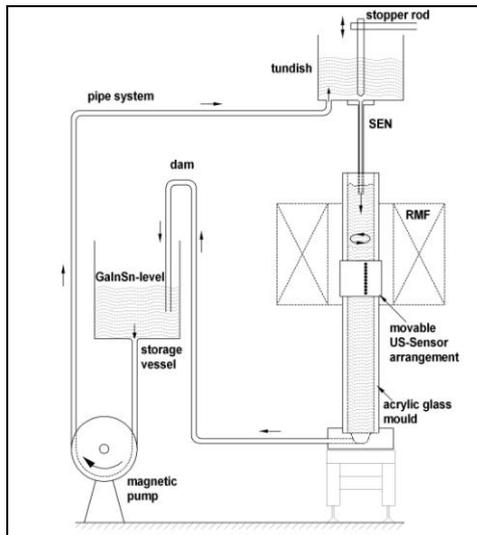
Fig. 1: Schematic view of the experimental setup showing the test section and the liquid metal loop
